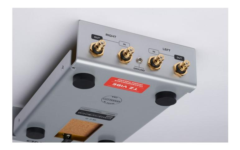
Place the **TZ VIBE** near the turntable. The turntable signal is applied to the two centrally located RCA jacks on the back panel. Often there is a ground wire coming from the turntable. Connect it to the grounding screw in the center of the back panel. The output of the **TZ VIBE** goes to a line-level input on your preamp or integrated amplifier.
