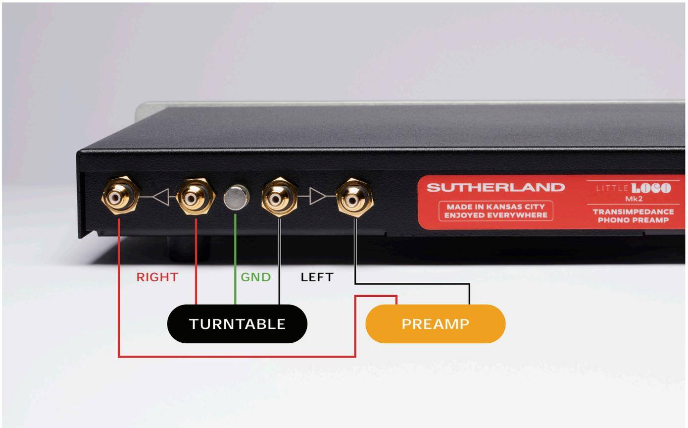
Place the **little LOCO Mk2** near the turntable. The turntable signal is applied to the two centrally located RCA jacks on the back panel. Often there is a ground wire coming from the turntable. Connect it to the grounding screw in the center of the back panel. The output of the **little LOCO Mk2** goes to a line-level input on your preamp or integrated amplifier.
