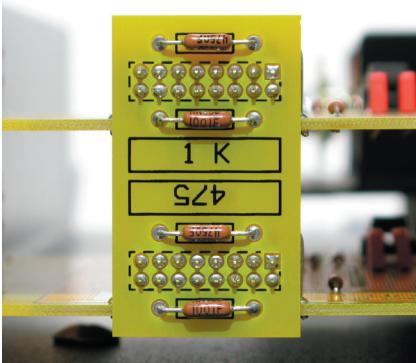
**A blank plug-in board is furnished. Any desired loading resistor and/or capacitor can be soldered to it. Install identical values in both the upper and lower positions. i.e. same values for each preamp channel.**
