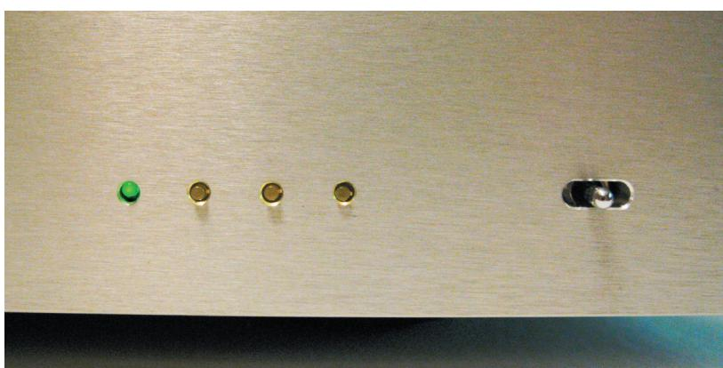
Move the momentary toggle switch to left to remove ON time. Each time it is moved, one hour will be subtracted from the remaining operating time.
